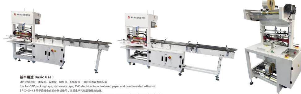
ZF-X400-XT is used to connect with the automatic slitting machine to realize automatic produce and packaging.
