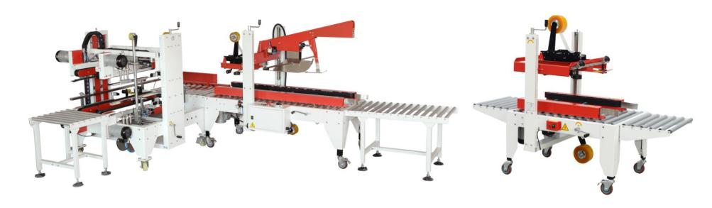
配套在全自动包装机后面实现自动封箱,大大节省了人工,降低了劳动强度,提高了生产效率。 This product is installed to the automatic packaging machine to achieve automatic sealing, greatly saving labor, reducing the labor intensity, and improving the production efficiency.
